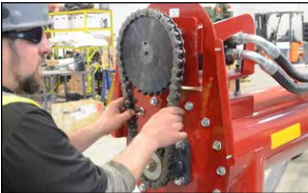
Fig 36 - Inspect chain and sprockets
