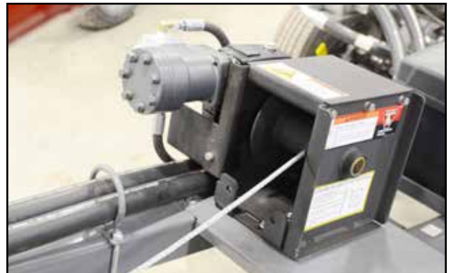
Fig 15 - Hydraulic winch for tube lift
