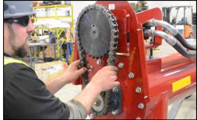
Fig 27 - Inspect chain and sprockets
