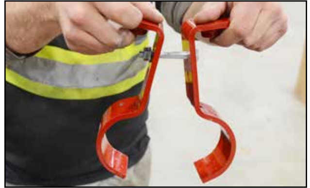
Fig 45 - 2 inch bolt joining the brackets
