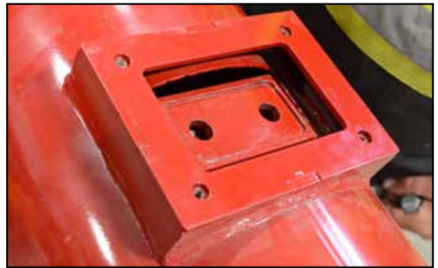
Fig 46 - Hanger bearing with Spacer Cover Plate
