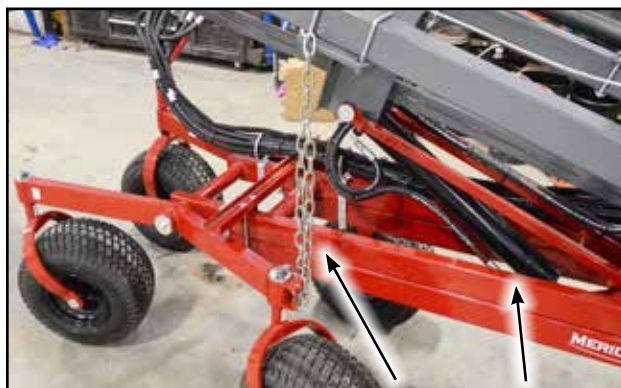
Fig 17 - Walking Beam transport chain and lift cylinder
