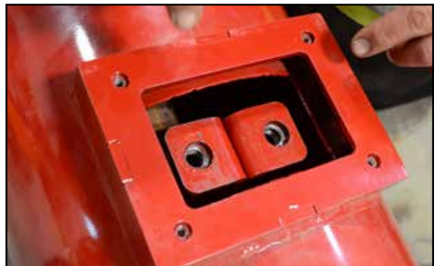
Fig 44 - Hanger bearing without covers
