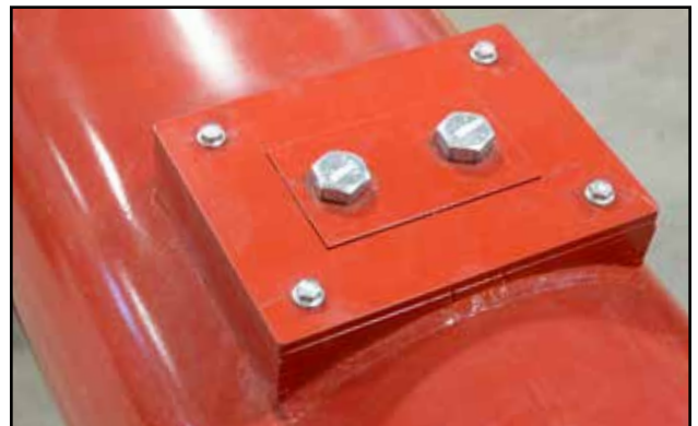
Fig 47 - Cover Plate covering Hanger Bearing
