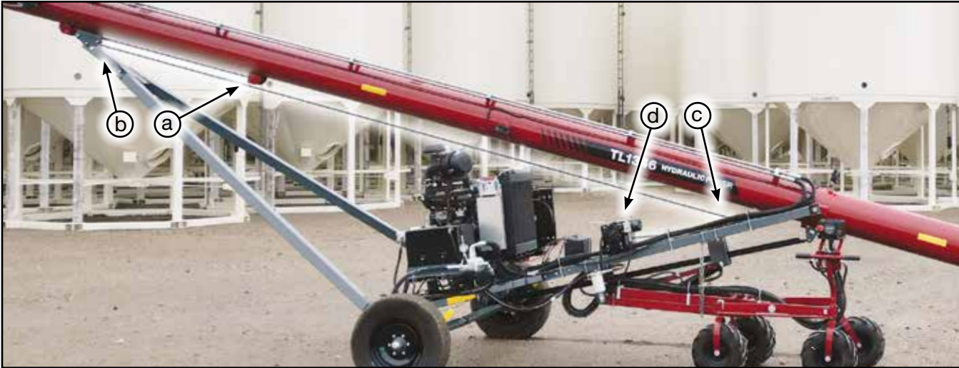
Fig 30 - Winch cable route
