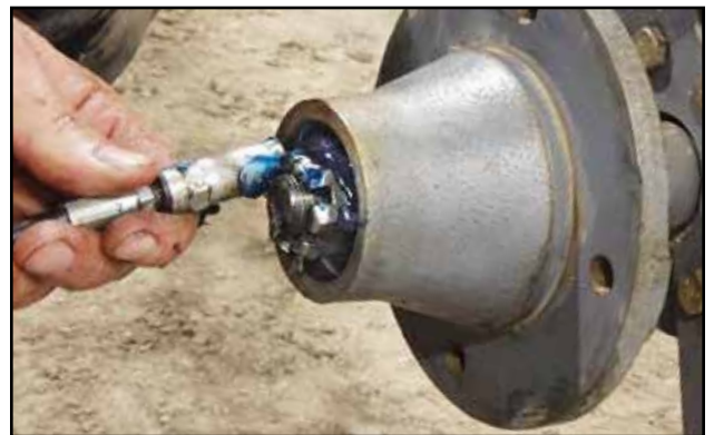
Fig 39 - Fill hub with grease
