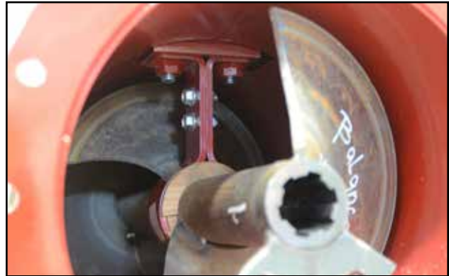
Fig 42 - Hanger bearing installed inside tube
