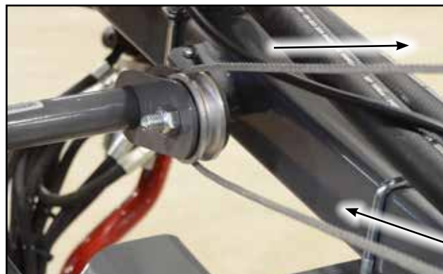
Fig 32 - Cable roller on main frame
