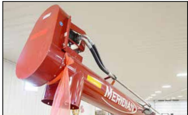
Fig 12 - Hydraulic drive for auger flighting
