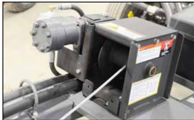
Fig 31 - Cable in winch spool
