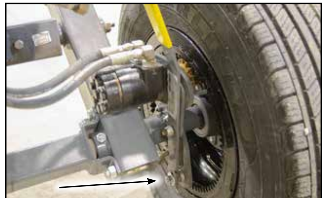
Fig 38 - Flange nut at bottom of assembly
