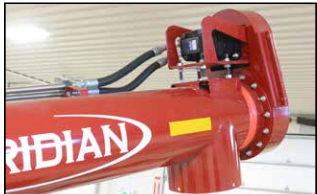
Fig 13 - Discharge-end hydraulic drive
